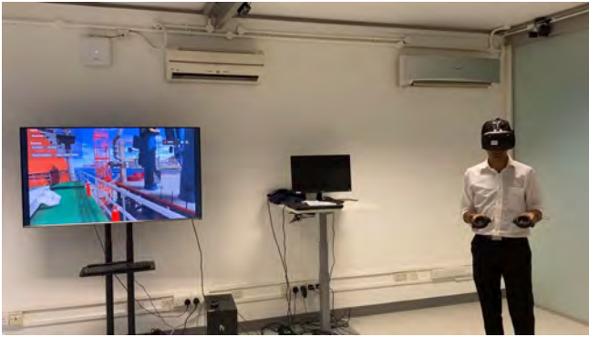
Figure 4. Trainee is wearing a head-mounted VR display and holding a pair of controllers which act as virtual hands in the virtual world. The monitor mirrors the scene seen by the trainee via his VR HMD.
