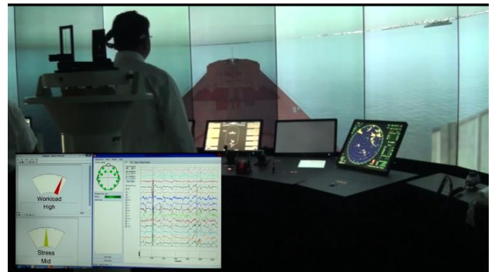
Fig. 11. The EEG-based human factors study experiment.
