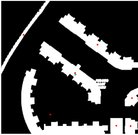
Fig. 11 Result of removing small objects and noise. Red dots are the centroids of contours and green dot is the image center
