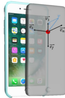
Figure 3: Directions of normal force, texture force and friction force.
