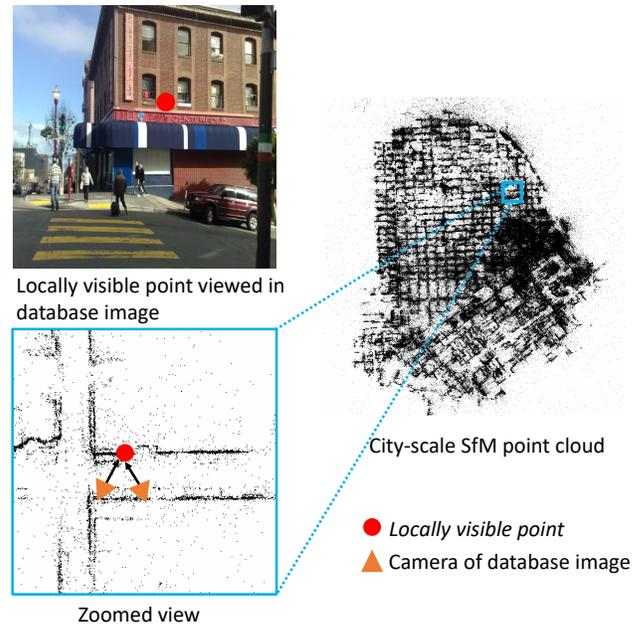
Fig. 3: An illustration of a *locally visible point* in the San Francisco dataset [4]. A *locally visible point* (red) is observed by nearby cameras (orange) of the database images.
