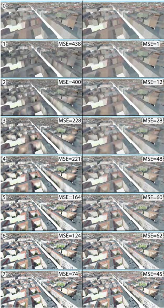
Figure 7: Frame captures of the Berlin (atlas) scene comparing direct mipmap sampling and our color blending method. *Left column*: Sampling the sparse image directly. *Right column*: Blending sampled colors in the sparse image with original mesh colors (shown in frame 0) stored in the City Colormap. Frames 1 to 7 indicate progressive sampling from the base sparse image mipmap level. The mean squared error (MSE) between the current and the previous frame is indicated.
