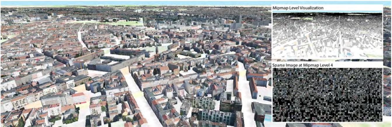
Figure 1: Rendering of the Berlin city dataset. 13.7K texture mipmaps are loaded and cached in the sparse image at a rate of 56.6MB/s. *Top inset:* The resolutions of loaded texture mipmaps are visualized as grayscale (i.e. lighter gray indicating higher resolution). *Bottom inset:* The sparse partially-resident image showing the cached level 4 texture mipmaps.
