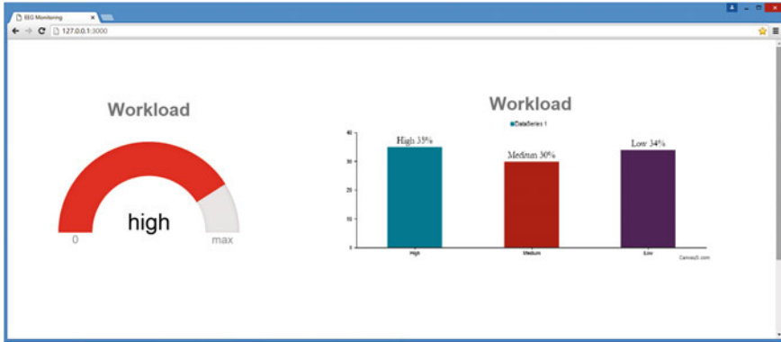
Fig. 5 Screenshot of EEG-based workload monitoring system. Left meter shows that current workload level is high. Right diagram shows overall distribution of different workload levels during the task performance
