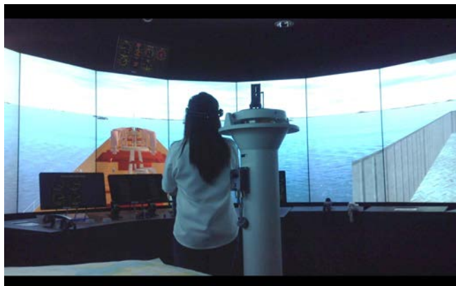
Assessing the cadet's emotional workload at the Maritime Academy's virtual bridge simulator with Fraunhofer Singapore's non-invasive, real time EEG based system
