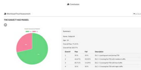
Assessing the cadet's emotional workload at the Maritime Academy's virtual bridge simulator with Fraunhofer Singapore's non-invasive, real time EEG based system
